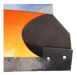
6. Verify the plow's cutting edge is on the ground. Hold the rubber cutting edge tightly against the ground, the Pro-Wing and plow's cutting edge. Mark location of the two holes in the bottom of the Pro-Wing on the rubber cutting edge from the rear and drill two 5/8 holes. Secure the rubber cutting edge to the Pro-Wing using ½" carriage bolt, 5/8" flat washer and nuts.
