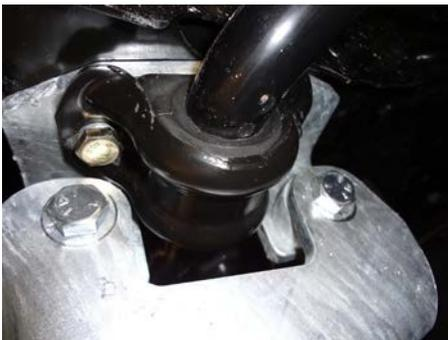
8. Fasten the spreader bar (1a) and the thrust arms (13)(14) to mounting brackets (11)(12) using 5/8" x 2 1/4" bolt (15), 5/8" lockwasher (16) and 5/8" hex nut (17). The spreader pin hole should be located 14 1/2" (+/- 1/2") of the ground.
