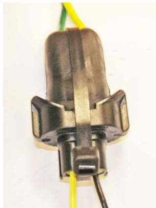
Apply grease and connect the rubber plug to truck harness connector using zip ties as shown above.
