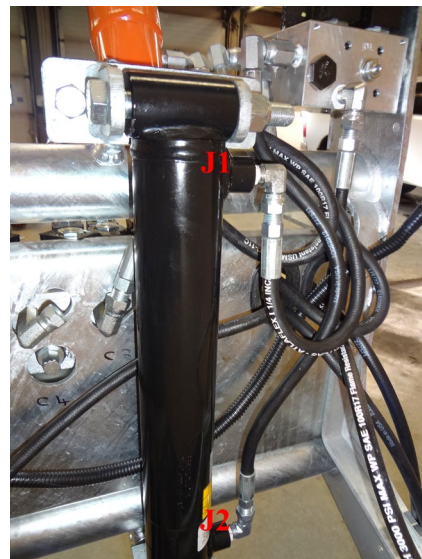
Jack hose installation (18” hoses)
