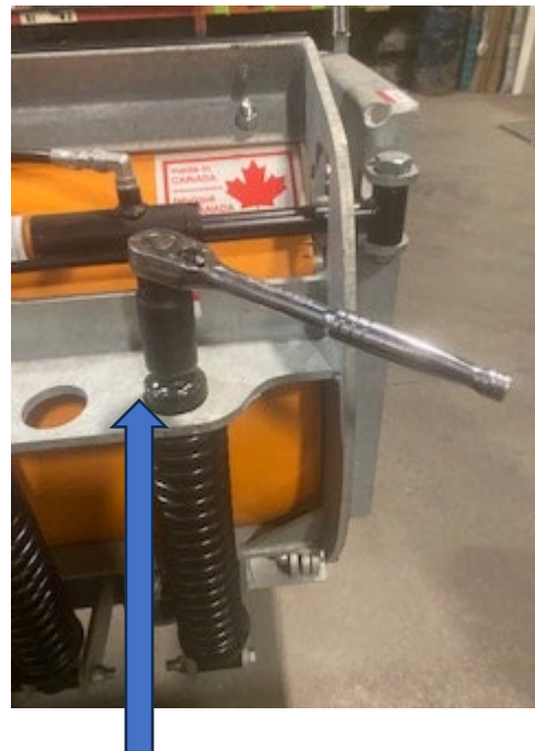
Use a socket 1 – 1/8" and turn it counterclockwise to compress the spring. After compressing spring, use 1-1/8" wrench to tighten the nut (turn it counterclockwise)
