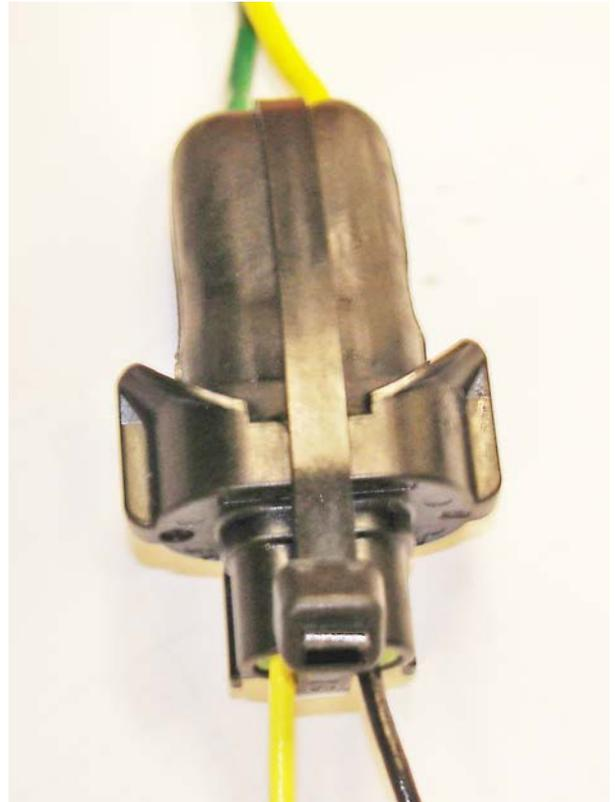
Apply grease and connect the rubber plug to truck harness connector using zip ties as shown above.
