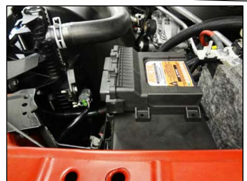
-plug the harness in the control module; install module on the fuse box
