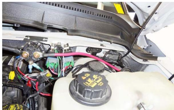
6. Slide Dummy Plug (15) over power cable (9) and ground cable (8) and route through grille of truck leaving sufficient length to attach to the cable and plug assembly (7). Secure the red power cable (9) to the large terminal on the solenoid and the black ground cable (8) to the negative terminal on the battery. (Drawing 1)
